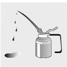
**Severe oil and grease marks** can be removed with alcohol based products, including methylated spirit and isopropyl alcohol or other solvents such as acetone. These products are not a corrosion hazard to stainless steel.
