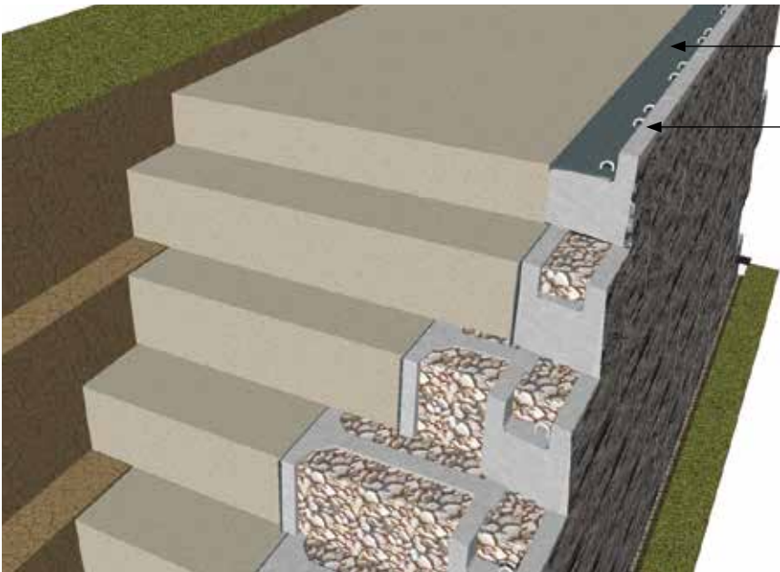
Clean stone or approved Backfill materials between extender units and inside hollow cores
