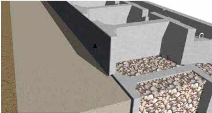
Filter Fabric placed behind extender units
