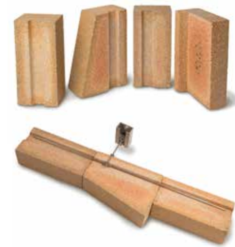
The special shape bricks were made by Bowral Bricks. From left: Centre Rebate, K Brick, Offset Rebate and L Brick. Not shown is the Solid Brick. A specially-engineered wall tie keys into the rebate and anchors the bricks to the inner steel wall, restraining the brickwork until the mortar hardens.
