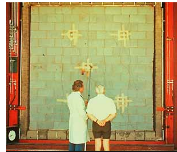
Figure 4.1 External Face of Typical Fire-Test Panel
