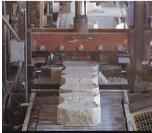
Retaining wall blocks being split on a special splitter to give a profiled face
