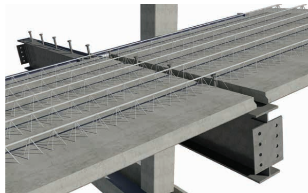
Figure 2 – Integration with steel framed structure.
