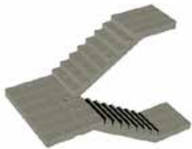
1 U Shape Stair Single Middle Landing
