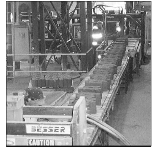
Figure 2.14 Cured Blocks on Machine Pallets being Transported to the 'Cubing' Machine after Unloading from the Kilns
