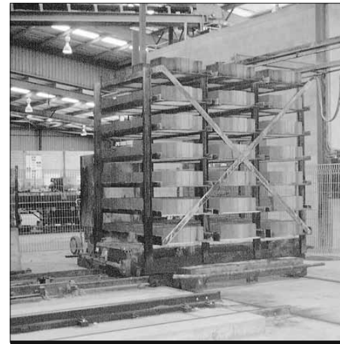
Figure 2.13 Automatic Rack-transfer Car System, Handling Loaded Racks to and from Curing Chambers
