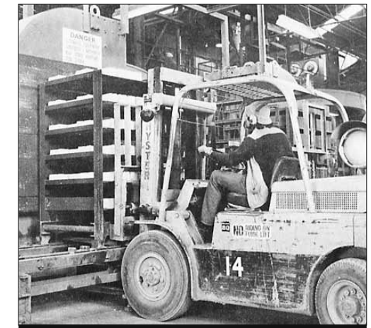
Figure 2.12b Forklift Truck Handling Racks of Blocks from Automatic Loading and Unloading Equipment, to and from Curing Chambers
