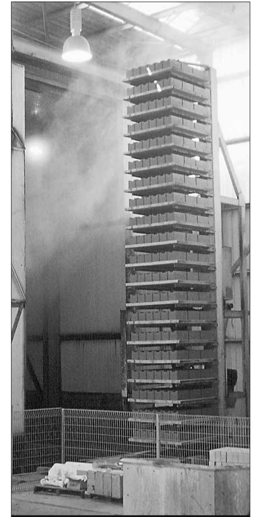
Figure 2.16 Low-pressure Installation with automatic Handling of 20-High Racks
