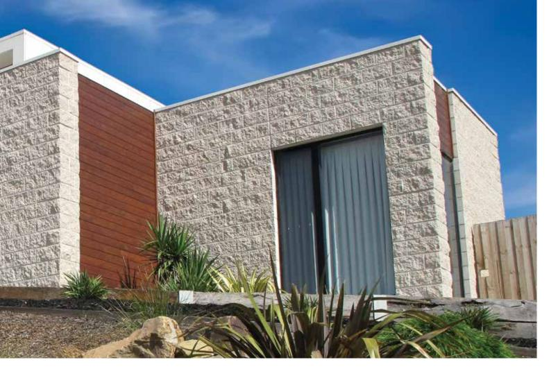
Although the building is clad in a variety of materials, the solid base of split-face concrete masonry predominates to the street, complementing the cedar panelling. The upper level is clad in composite fibre-cement panels, cedar and corrugated steel.
