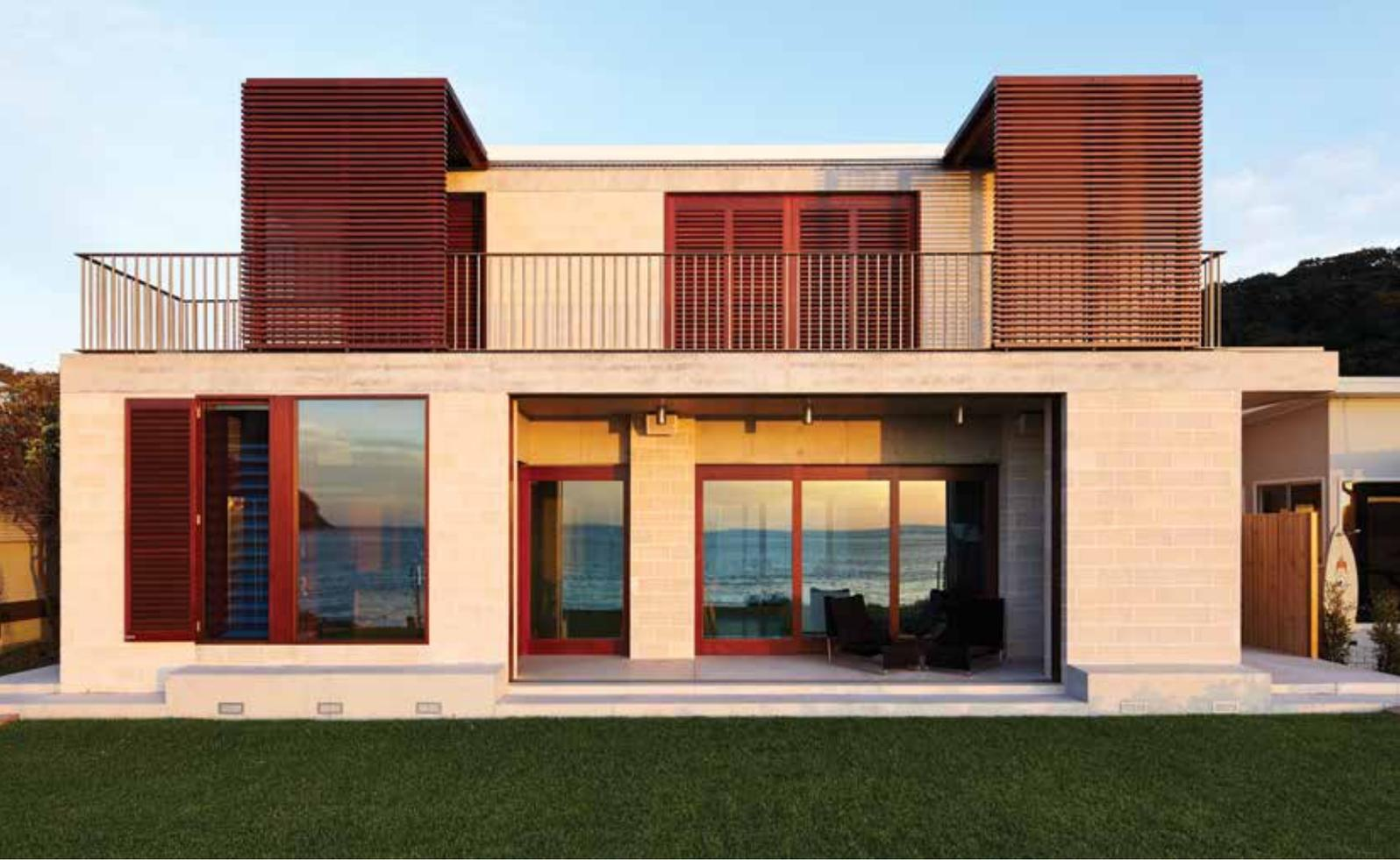
and Polished. These blocks are available in many of the same sizes as their industrial grey concrete masonry cousins, but with a much finer surface finish and contemporary colours.
