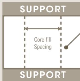
Single steel reinforced and fully grouted cores.
